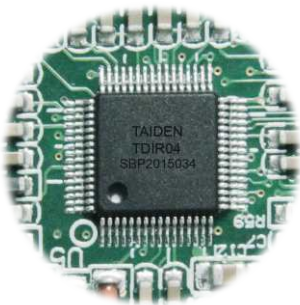
TAIDEN TDIR04 Digital Infrared Processing Chip
