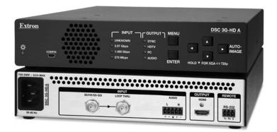
The Extron DSC 3G-HD A is a high performance scaler that converts incoming 3G-SDI, HD-SDI, and SDI video signals to HDMI. It accepts SMPTE video resolutions and generates HDMI output rates up to 1920x1200, including HDTV 1080p/60 and 2K.
