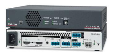
The Extron FOX II T HD 4K is a transmitter for long haul extension of HDMI video, multi-channel audio, RS-232 control, and IR control signals over fiber optic cabling. It provides a variety of new integrator-friendly capabilities, including support for 4K resolutions. Use of the FOX II T HD 4K simplifies the integration of 4K HDMI sources in a fiber optic AV system.
