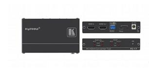
FC-17 is a versatile HDMI 4K@60Hz (4:4:4/4:2:0) converter tool. FC-17 can convert from 4:4:4 to 4:2:0 color sampling and offers EDID management via a user-friendly Windows application. It also enables inter-operability between HDCP 2.2 and HDCP 1.4 systems. FC-17 acts as an HDMI extender that equalizes and reclocks TMDS data before re-transmitting, thus increasing the HDMI cable range from the output
