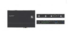
DIP-22 is an extended reach 4K@60Hz (4:2:0) HDBaseT transmitter and Step-in commander for DisplayPort (DP++), HDMI and VGA video input and unbalanced stereo audio input. It provides full room automation including control of lights, screens, shades and many other exciting options. In addition, DIP-22 accepts Ethernet and serial data input signals for control
