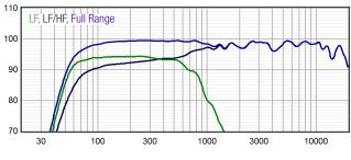
Axial Processed Response (dB) The axial magnitude response with processing
