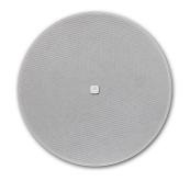
The CM20DT 6.5" two-way built-in loudspeaker can be used in 16 ohms or 70/100 volt modes. The high-quality 70/100 volt transformer is equipped with an easy tapping sticker with clear colour indication. The transformer colours are aligned with the cables connecting the Apart Quick Fit connector, a handy installer connector via push terminal
