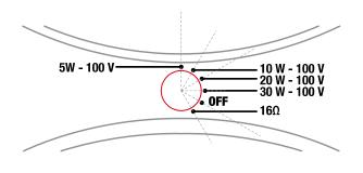
Note: if the rotary switch is set to the OFF position, the loudspeaker will be muted.
