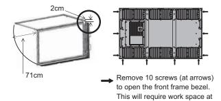
(\*3) The front frame bezel is hinged to the cabinet. 2cm of space is required for opening it as illustrated.
