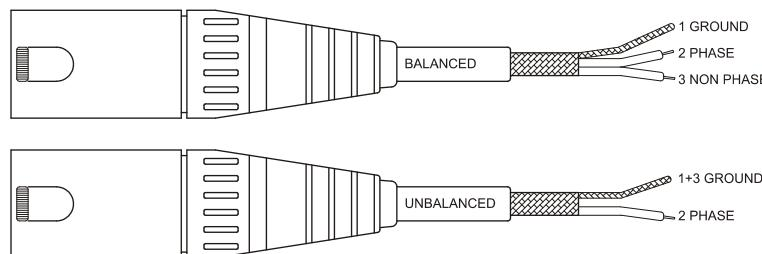
The "STACK" (39, 40) are in parallel with the inputs and are used to supply the same "INPUT 1", "INPUT 2" input signal to other amplifiers or sound systems. This signal output connectors are of jack 1/4" type. The pin assignment is as follows:
