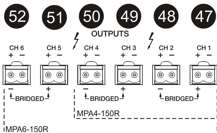
Connect the terminal blocks securely, removing the cable cover 5÷7mm from the end.
