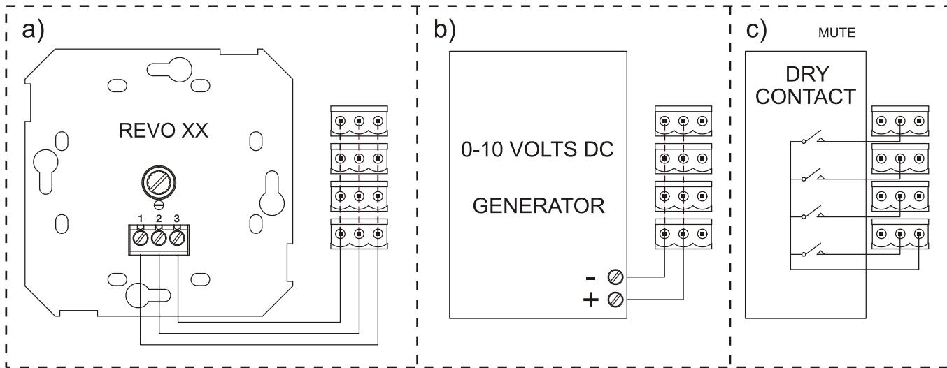
NOTE: it is possible to connect a maximum of 16 inputs to one control potentiometer. It is necessary that the ground terminals of all amplifiers are connected.
