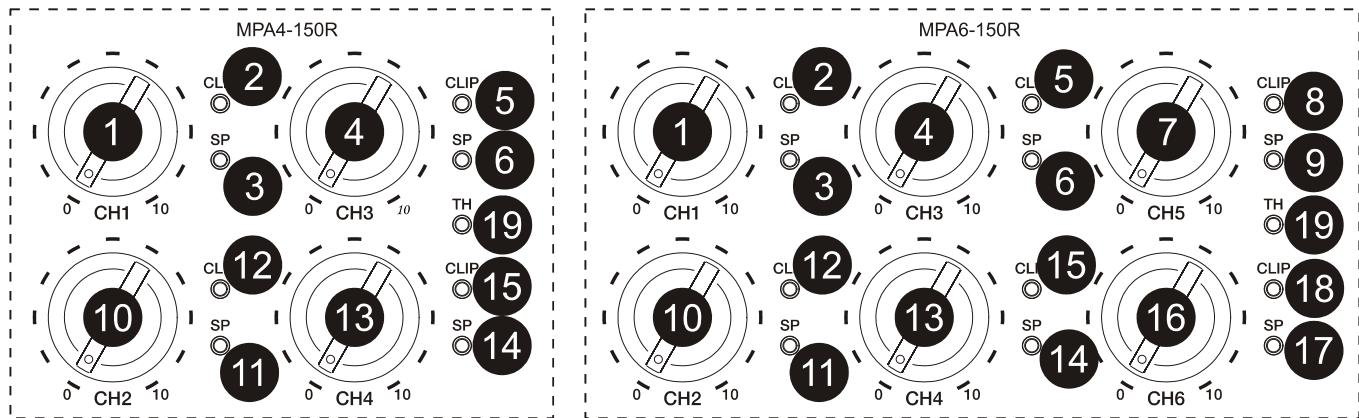
These attenuators allow the connection of different mixers, an independent volume control and the connection of speakers not able to handle the amplifiers maximum output power, thus avoiding the risk of damaging them with the mixers or preamps volume control.
