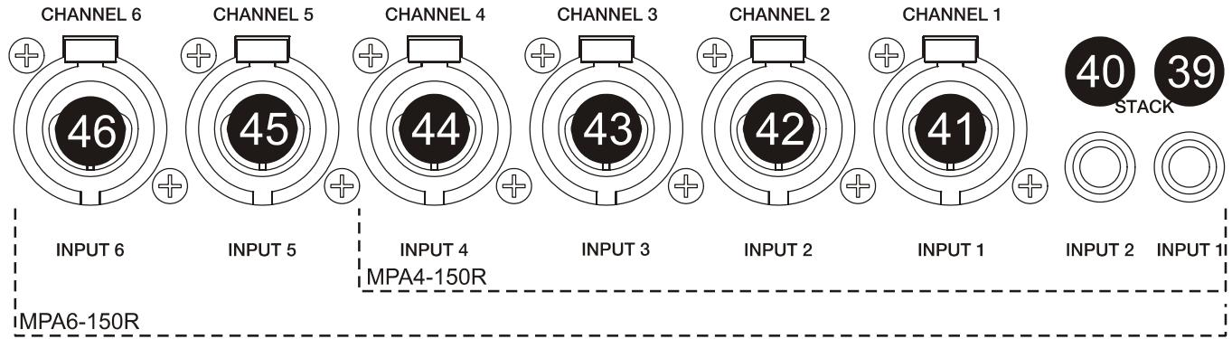
The signal input connections (41, 42, 43, 44, 45, 46) are electronically balanced XLR-3 sockets, with input impedance higher than  $20\text{k}\Omega$  and a nominal sensitivity of  $0\text{dBV}(1\text{V})$ . Pin assignment:
