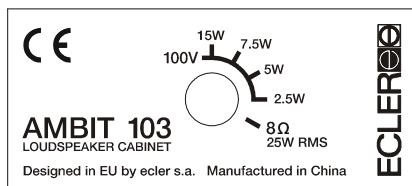
The AMBIT103 has 4 power handling levels for the 100V line. Depending on the intended use, the speaker output can be attenuated more or less. In the zones where sound intensity should be low, place the switch in the 2,5W or 5W position. If sound intensity should be high, place the switch at 7,5 or 15W.
