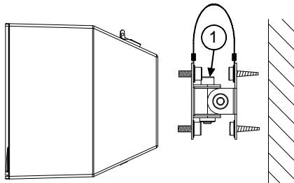
The AMBIT103 has 4 nuts inserted in the rear at a standard diagonal distance of 60mm, to permit the safety sling screw to be housed and to be coupled to a standard bracket.
